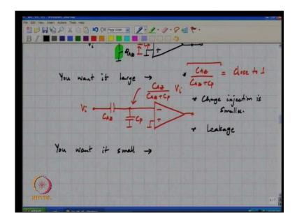
So, during the amplify phase the effective circuit looks like this, so this is C A Z, this is C p and this is the preamp, and this is V i, so what is this voltage, so this is nothing but, C A Z by C A Z plus C p times V i. And is therefore...
