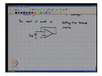
During the autozero phase, please note that the equivalent circuit is this, so the amplifier has to drive a load equal to C A Z, so if C A Z becomes too large, what happens?
