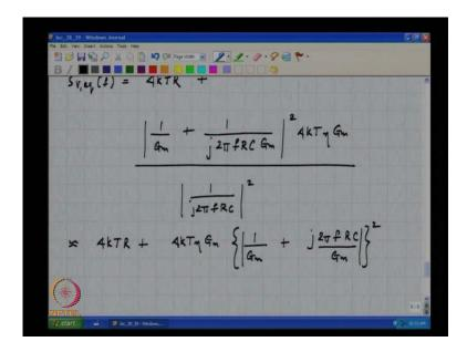
So, clearly S v equivalent of f is nothing, but you divide throughout by this factor, and when you divide this goes away. So, you get 4 k T R this makes sense because, the noise source corresponding to the resistor is at the same place as the equivalent noise source that you are trying to find. So, it is no surprise at all that 4 k T R appears all right, the next thing is this factor divided by ((Refer Time: 25:08)) this.
