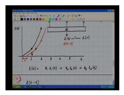
So, if the loop delay is tau and tau is less than 1, the ideal output of the loop filter is probably something like this, and why does this make sense ((Refer Time: 04:52)) this is the pulse response of the ideal loop filter and why does this make sense.
