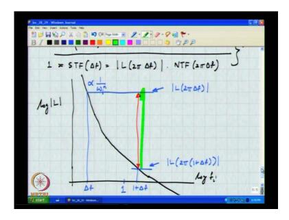
If you have a high order loop filter, at low frequency, it will behave like... If you have an n-th order loop filter; at low frequency, how will it behave like?
