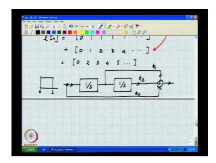
So, in general, let us say you have 1 over s. And, in general, the loop filter should be of the form? At low frequencies, it must be of the form 1 by s square. So, in general what do you think will be the form of the loop filter transfer function?
