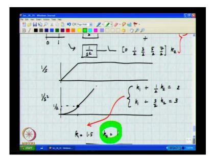
k 1 plus half k 2 is 2. k 1 plus 3-halves k 2 is 3; from which we obtained k 2 is 1. You subtract the two equations. k 1 goes away and k 2 simply becomes equal to 1. And, what about k 1?
