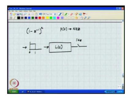
So, we were done with the first order system; now, let us try and realize a noise transfer function of the form 1 minus z inverse the whole square. And, the problem as I mentioned is to determine L of s such that this noise transfer function is realized. And, what all do I need to know?
