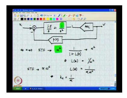
Let me just draw the loop filter as 1.5 by s plus 1 by s square is the loop filter. And, this is p of t. So, why does it make sense that, this coefficient is 1?
