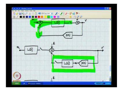
So, like in the first order example, we can manipulate this system into an equivalent mathematical model by separating the discrete-time and the continuous-time parts. We pull the loop filter out in this fashion. So, all I have done is move the loop filter through this summer like this; and, also pull the sampling operation out of the loop, which results in this diagram. Then, we identify this animal with L of z. Therefore, one ends up with this equivalent of the modulator.
