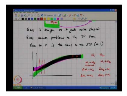
So, the spectrum here is consists of the input plus some shape noise, right. And, e DAC is a non-linear function of this sequence which has got this spectrum, right. If you take something like this and pass it through a non linearity what do you expect you will get? If you take a sinusoid and pass it through you will get harmonics, very good. So, in so, you start to see harmonics of the signal and what else do you think you will see, what about noise.
