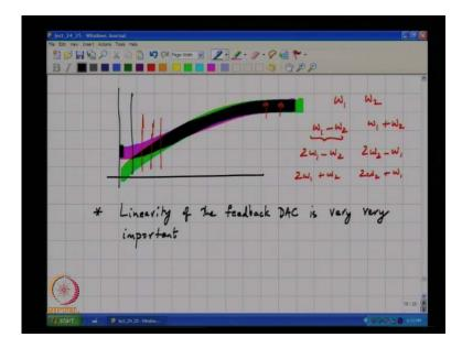
So, linearity the bottom line therefore; is that linearity of the feedback DAC is very important, because the errors in the DAC output directly it appear, as if they are being added to the input. And, therefore appear directly at the output of the modulator. Whereas errors in the flash I mean the in the A to D converter thresholds are not really a problem because they get noise shaped, is this clear. So, this is regarding a multi bit
