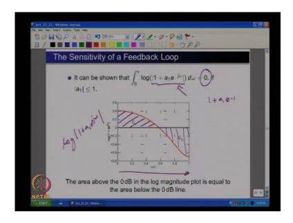
Now, it turns out that it can be shown that if I evaluate the integral from 0 to pi of the log of the magnitude of a term 1 plus a 1 e to the j omega from 0 to pi. Then, this turns out to be equal to 0. You understand? Let me repeat this again. I have a term 1 plus a 1 e to the j omega. In other words this is nothing but 1 plus a 1 z inverse evaluated on the unit circle, right; I find it is magnitude only take the logarithm and integrate it from.
