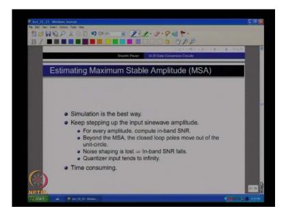
All right. Before, I go further I just like to mention you know how one might estimate the maximum stable amplitude of a modulator in practice. This is obviously, something which is very relevant, right. So, simulation is the most reliable way of doing it, right; in the given that doing this analytically, it can be a very messy effect. So, one thing you could do is put a sinusoid with some amplitude. Look at the state variables inside, if none
