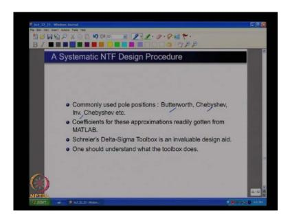
So, the systematically design an NTF, what? one realizes is that a noise transfer function is nothing but a high pass filter. So, the job of designing a noise transfer function is analogous to that of designing a proper high pass filter. But can any high pass filter be a noise transfer function.
