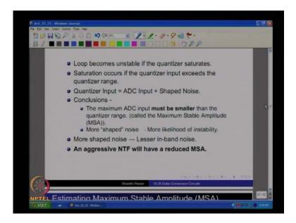
So, again to retreat the maximum ADC input must be smaller than the quantizer range right that this is the; so, called u that we have been talking about. And, which has more shaped noise; then, it means that there is more likelihood of instability. And, as we have just seen now we made a passing observation, that the more the shape noise the smaller seems to be the.
