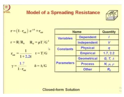
The variables, constants and parameters of the model were as listed in this figure. The empirical constants of 1.7 and 2.2 were necessary to improve the continuity and accuracy properties of the model.
