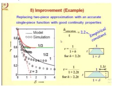
Now, let us consider replacing the 2-piece approximation with an accurate single-piece function with good continuity properties. Note that in the process of incorporating the saturation resistance we have also incorporated the t/G dispersion because the value of the saturation resistance depends on t. So, as t changes the saturation resistance also will change. So, in 1 shot we have incorporated resistance saturation.
