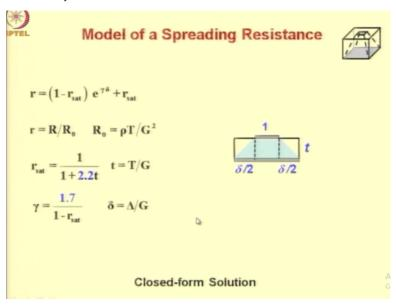
Now based on this, we obtained the model shown here after attempting the improvement of the basic model based on the constant angle current spreading approach.
