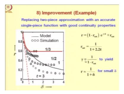
Now if expression which is again empirically determined which has the shape is given by this formula r=1 - saturation value of r into exponential of - gamma into delta+r sat. Note that as delta turns to infinity this quantity goes to 0 and r becomes r sat. So, that is how you get this constant segment. On the other hand, for delta = 0 this quantity becomes unity the r sat cancels and you get r=1 that is how you get this value.
