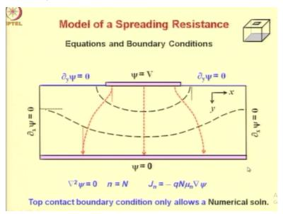
Next, we considered equations and boundary conditions. The equations were Delta square psi = 0. Electron concentration = doping concentration and electron current density = - q, doping concentration into mobility into gradient of psi, because the current was only due to drift. These equations followed from the qualitative model. Similarly, the boundary conditions shown here also followed from the qualitative model.
