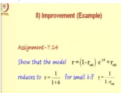
An assignment shows that the model r = 1 - r sat into e power - gamma delta+r sat reduces to r = 1/1+delta for small delta if gamma = to 1/1 - r sat. Let us come to the final step of parameter extraction. First we will make some general comments about parameter extraction and then we will illustrate the procedure of parameter extraction using our spreading resistance example.
