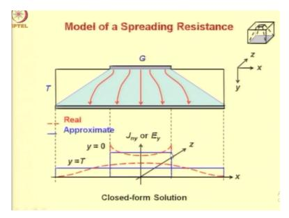
Therefore, we went in for a closed-form solution in which the following assumptions were made. Firstly, that the current spread at a constant angle from the top contact to the bottom contact. And secondly the distribution of electron current density or electric field normal to the horizontal cross sectional area of the device was assume to be uniform over the current flow cross section.
