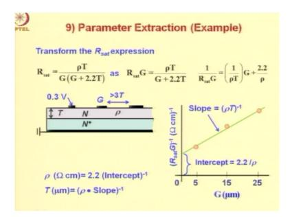
So, transform the R sat expression given here as R sat into G = rho T/G + 2.2 T. Now this is an important aspect in parameter extraction. The model expression will have to a transformed so that you can plot the data in a simple graph preferably as a straight line. So that is the intension of transformation. So, we have moved G to the left hand side and taken the product R sat into G. It turns out to be of this form.
