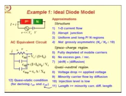
Let us look at the AC equivalent circuit based on the same diode model. So in this case, you are applying a small signal voltage, which is much less than the thermal voltage and this small signal voltage is superimposed over DC voltage. You have a DC current or which a small signal current is superimposed. The relation between small signal current I and small signal voltage V is given by this equivalent circuit, which has a resistance in parallel width, two capacitances.
