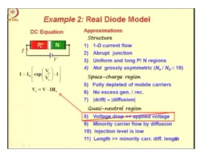
To look at the approximations associated with the real diode model let us begin with the ideal model. So this is an ideal diode equation and these are the set of approximations associated with an ideal DC equation. The real diode model is obtained by dropping the various approximations one by one. For example, if you drop the approximation that there is no voltage drop across the quasi-neutral region then the modification that happens to the ideal diode equation is as follows.
