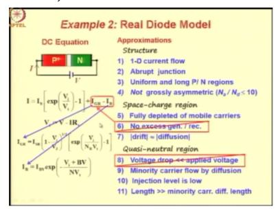
The thermal generation recombination is given by IGR = ISR which is reverse current due to generation recombination multiplied by 1 - the internal voltage that is the voltage across the space-charge region divided by the built in potential of the junction that is V suffix j multiplied by exponential of Vi divided by NR Vt where NR is an ideality factor related to generation recombination -1.
