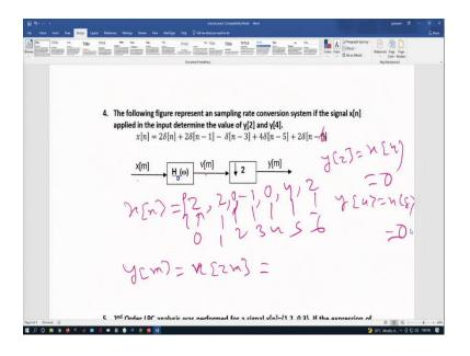
Now, let us look at question number 2 4. What did I say? The following figure represents the sampling rate conversion system. If the signal x n is applied in the input, determine the value of y[2] and y[4]. So, what is x[n]? x[n] What is the sampling repetition? 2 is the 0th sample, so I know 2 is the 1 sample, and minus 1 is the third sample, so that means 0 1. So, it is minus 3; that means 0 1, then 1 0 will be there, and then minus 1 is okay.
