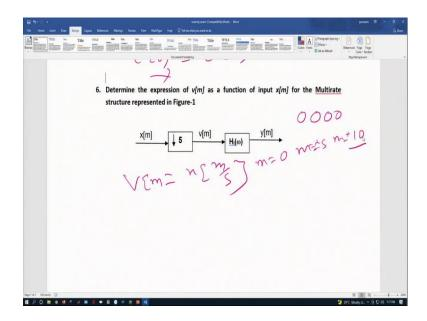
Then, I will determine the expression of a v[m] as a function of input x[m] in multi-rate signal processing. So, what is v[m]? v[m] is nothing but a x[m] m by 5. So, what is required? So, I have to 40 is inserted between 1 to 5th simple 11 to 2nd sample, where m is equal to 0, m is equal to plus minus 5, m is equal to plus minus 10 like that ok.
