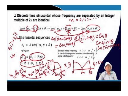
The next one is a discrete-time sinusoidal whose frequencies are identical and separated by an integer multiple of  $2\pi$ . Before that, let me give you the back concept in the sampling; what is the concept? Suppose I have a baseband signal like fm, this kind of structure. If I sample this signal with sampling frequency Fs. So, what is the frequency response we have drawn for the frequency?
