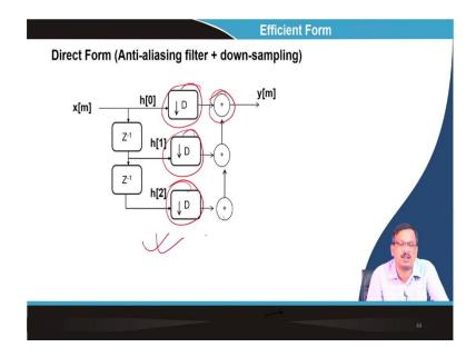
So, this D-down sample can also go inside. So, I can say that instead of the whole filter after downsampling, I can put this downsampling inside that direct structure. So, what will happen? That means it will reduce the sum complexity, ok? So, that is the efficient implementation of a direct form of the filter, or, I can say, a decimation filter similar to a downsampling filter.
