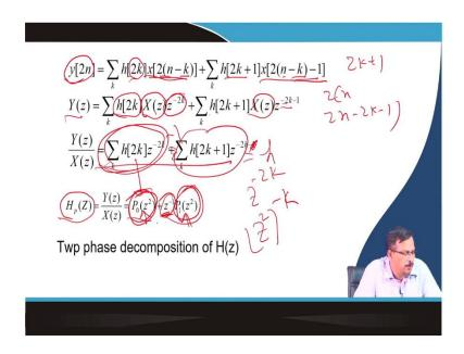
If I say, this is the y[even] y[2] n. So, it exists 2 k 2 n minus 2 k, and this is odd 2 k plus 1 is odd. So, it is nothing but a 2 into n 2 n minus 2 k plus 1. So, that is this one. So, I can say y(z) is equal to h[2k] z to x(z). This is nothing but a x(z)  $z^{-2}$  k. similarly, this is nothing but an x(z)  $z^{-2}$  k minus 1.
