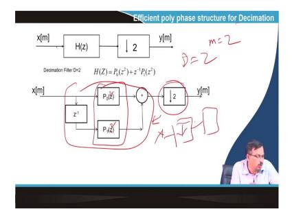
Similarly, let us say m is equal to 2. This one ok. So, this is a decimator, and decimation factor D is equal to 2. So, I decomposed that filter into 2 poly phase form and decimated it by factor 2. That means this filter will not use that discarded sample. So, this will be z square.
