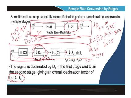
Now, there is another problem. That is called sampling rate conversion by stage. Instead of single, let us say this is a single-stage sampling rate conversion. This is a single-stage poly. So, single-stage sampling rate conversion. So, downsample by factor D in a single stage.
