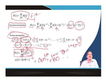
So, if I want to put it in a generalised form, let us say H(z). This is my FIR filter, ok? So, now, H(z) is equal to. So I can break even and odd terms. So, when I break it even and odd, it is nothing but a Po(z) square plus  $z^{-1}$  P1(z) square. So this is called 2-phase decomposition.
