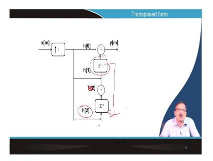
It can be said that instead of z, I can also put the z here. So, this is not there. So, this will be there. So, I can put the z here. So this is called a transpose form of that implementation.
