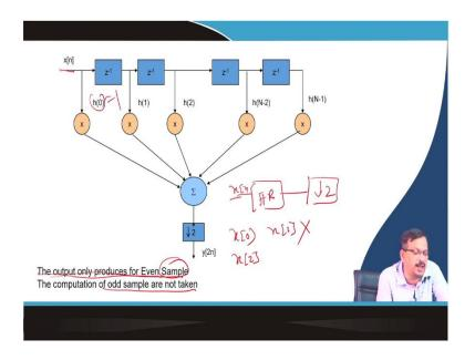
So, what is poly-phase implementation? So, let us say I have a filter x[n], x[n] that passes through an FIR filter and then downsamples by 2; let us say this is my system diagram. So, what I said is output is only produced for the even sample, and computation of the odd sample is not taken because I know I will take x[0], then I will take x[2], not x[1], because x[1]. I am discarding it as a downsample by 2. So, even sample output is produced, and odd sample output is not produced.
