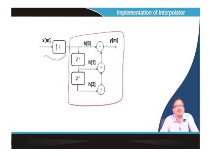
Similarly, upsampling followed by a filter can be implemented again using a direct form structure for interpolation or upsampling. So, it is nothing but a h[0]  $z^{-1}$ . So, delay and then multiply and sum.
