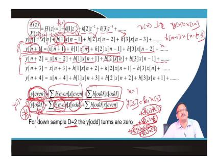
So, let us say write down that mathematical form. So, I can say y(z) by x(z), which is the filter called H(z), is nothing but a 1 plus z to the power 1 h[0] if the h[0] is equal to 1 then I can say it is 1 into h[1] into  $x(z)^{-1}$  or I can write h[0] also here. So, here will be h[0] ok.
