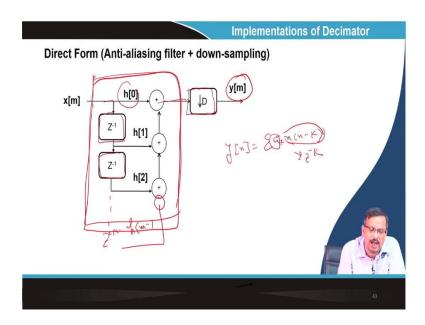
So, let us. So, what I said is that whether it is down-sampling or upsampling, this side is nothing but a filter. So, this filter is nothing but an FIR filter. If I say that, then the FIR filter can be implemented this way: the delay. So, what is an FIR filter? y[n] is equal to the summation of that a k into x[n-k].
