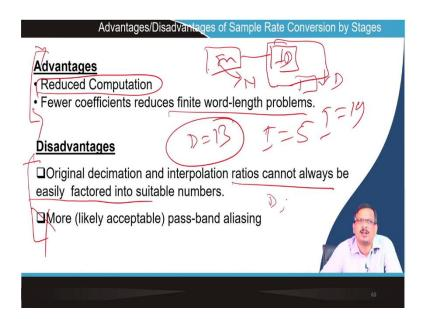
Similarly, for interpolation also that I can instead of single interpolation, I can say that upsampling by, let us say, up the sample, I is equal to, let us say, 50. So, first up the sample by 25, then up the sample by 2 possible. So, multi-stage sampling rate conversion. So, why do we use multi-stage? What is the advantage of using a multi-stage system? The advantage is the reduction of computation. I will show you.
