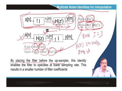
Let us say x[n]. So, this is the up sampler block diagram of an up sampler. So, I up the sample, then pass remove that image, multiple images keep the single image and then I get the y m. So, if I do this block diagram. So, what is V1(z)? V1(z) is nothing but an  $x(z^I)$  if it is up-sampling by factor i. And then what is y(z)? y(z) is v 1 x. So, x of z to the power I pass through the  $H(z^I)$ .
