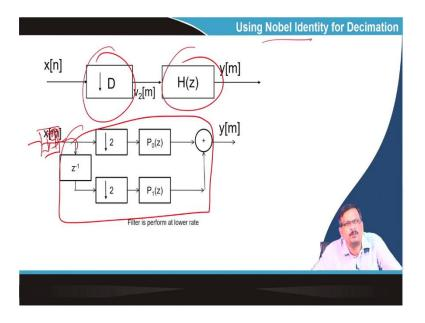
Similarly, decimation can be that if I use the Nobel identity here. So, I filtered and downsampled; the identity they said allowed me to downsample the signal and filter. So, I used Nobel's identity first down sampling, then filtering. So, I can do that with that one,
