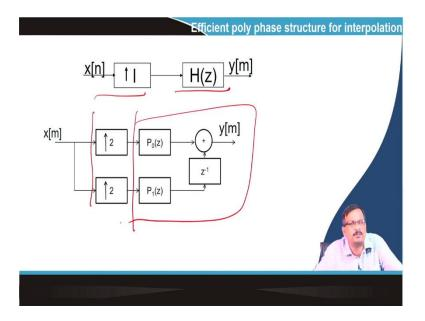
Similarly, for interpolation, upsampling and filter H(z) is implemented this way, you are doing poly phase filtering ok.
