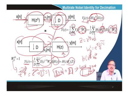
So, I can implement that FIR filter, whether it is HD or FIR filter, after that upsampling or before the downsampling, which is called an anti-aliasing filter and after it calls that removing of the multiple images of the signal. So, both can be implemented using the FIR filter.
