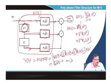
So, let us say I have a 3 phase, yeah. So, H(z) is equal to 3 phase decomposition I equal to 0 to 3 minus 1 z to the power minus I P I z to the power M, M is equal to 3. So, there will be a z-cube, ok? So, I can say H(z) is nothing but a  $z^{-0} Po(z)^3$  plus  $z^{-1} P1(z)^3$  plus  $z^{-2} P2(z)^3$ . So, how do I implement x[n]? So, this is x of. So, this is my H(z).
