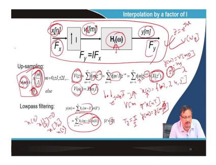
Let us say. So, I know that my interpolation filter in the upsampling block diagram looks like this x[n] Fx is the input sampling frequency v[m] and then,  $H(\omega)$  and y[m] Fy. This is my upsampling block diagram.
