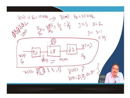
Let us say I have a signal x[n]. I have a signal x[n] sampling frequency of x[n] is equal to, let us say, 10-kilo hertz d. Write down the functional block diagram of a fractional signal sampling rate converter to convert to y[n] with the sampling frequency Fy is equal to, let us say, 25 kilohertz.
