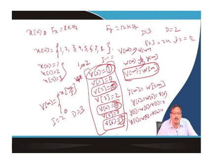
So, I have a signal x[n] x[n] whose sampling frequency is Fx is equal to 8 kilohertz. Now, I want to make it Fy, which is equal to 12 kilohertz. That means the up sample is 3 and the down sample is 2, with I equal to 3 and D equal to 2. An up sample is measured by 3; that means 8 are divided into 3, and a down sample is measured by 2. So, it is 24, and downsampling by 2 means 12. Ok, done.
