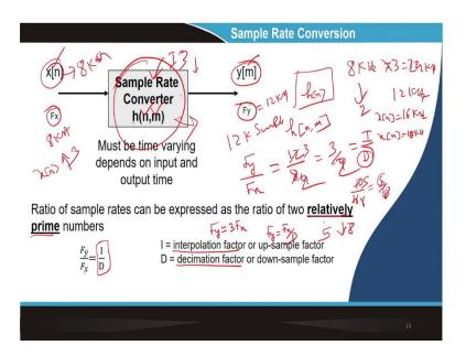
So, when I say the sampling rate converter, the sampling rate converter is nothing but x[n], which is the input whose sampling frequency is Fx. I want a y[n] as an output whose sampling frequency is Fy. So, the process of the system or inside that what I have to do for that whole system is called sampling rate conversion, or the system is called sampling rate converter.
