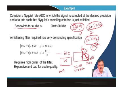
For the next example, I said that sometimes sampling decreases the complexity of the system. What is the example? Let us say I have an audio bandwidth. You know the audio bandwidth is 20 kilohertz, which is the maximum bandwidth of the audio signal perception of the human being; a human being can perceive audio up to 20 hertz. So, if it is 20
