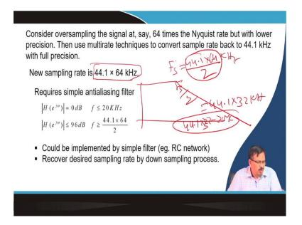
But let us say instead of designing this, I let us say instead of now my sampling rate is Fs instead of 40 kilohertz; I said 44.1 kilohertz. I said it is 44.1 into 64 kilohertz. So, 64 times, I up-sampled the signal. So, 64 times I upsample the signal; that means, once I do 64 times sampling, what are the Fs by 2 values? This is divided by 2, which is nothing but 44.1 into 32 kilohertz. So, if I say 44.1 into 32 minus 20 kilohertz. So, there is a huge long transition bandwidth.
