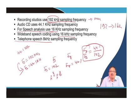
Let us give another example: if you go to any recording studio, you can see the recording studio uses 192 kilohertz sampling frequency for master voice. That means when the recording student studio records that audio signal for the master cassette. They use 192 kilohertz sampling frequency, but for any audio CD, the sampling frequency is 44.1 kilohertz. So, I have an F, which is 192 kilohertz.
