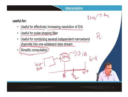
Similarly, in the case of upsampling or interpolation, it is useful for effectively increasing the resolution of the DA digital to analogue converter. So, suppose you know that I have an 8-kilohertz sampling frequency. I want an exact copy of that input signal when I want to convert to an analogue signal. So, if the number of samples within a time increases the efficiency or effect, I can say there is an increase in the resolution of the digital-to-analogue converter.
