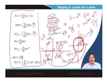
Now, when mapping the z-plane to the s-plane, whether this means that the transform is stable or not, what is the mapping of the z-plane to the s-plane? I am not going into details on this side, but I have already explained. Is that okay? So, what is z? Z is equal to e in the power sT. If you see that z is equal to e<sup>pkT</sup>, the position of the pole so, s is the pole position ok.
