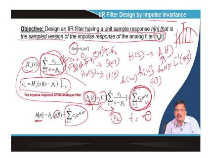
So, now, let us discuss about impulse inversion in the impulse<sup>-1</sup> method. So, what is objective? Design an IIR filter with a unit response; let us say if the H(s) is my Laplace transform, then if the h(t) is my time domain transfer function of the filter.
