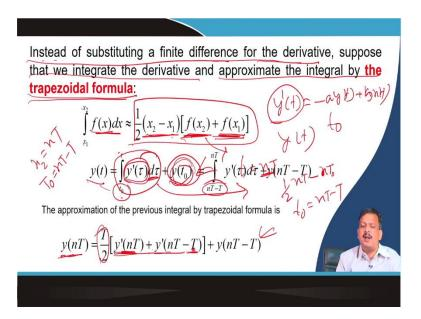
So, what is the meaning? Instead of subtracting a finite difference from the derivative, suppose that we integrated the derivative and approximated the integral using a trapezoidal format. So, the derivative is nothing but a here you can see; it is a difference differentiate. Instead of that, if I do the integrated so, I can say y(t) is equal to t 0 to t y prime t plus d t, so this is ok. Think about it.
