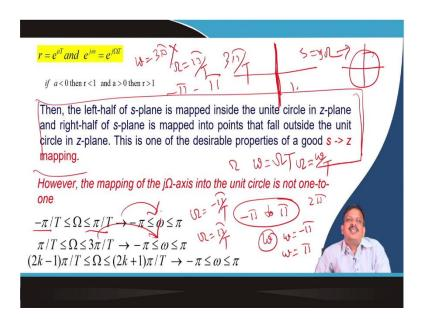
So, we see again that s z is mapping, so that is the mapping which I explain is written in here. So, the left-hand side s-plane plane poles are within the unit circle of the z-plane, and the right-hand side pole is outside the unit circle, and that pole is ok. Now, how the mapping of j  $\omega$  axis, how do I map the j  $\omega$  axis?
