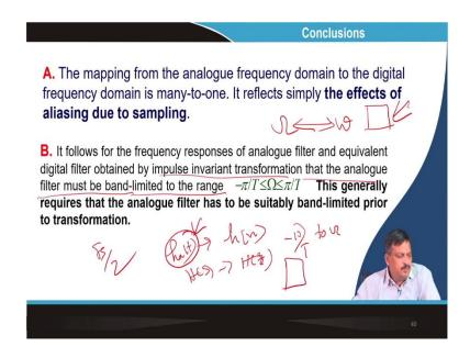
So, in conclusion, we can say the mapping from the analogue frequency domain to the digital frequency domain is many-to-one. It reflects simply the effect of aliasing because analogue frequency  $\omega$  capital  $\omega$ , discrete frequency small  $\omega$ , this mapping is many-to-one. It follows the frequency response of the analogue filter and the equivalent digital filter obtained by impulse invariant transformation that the analogue filter must be band limited.
