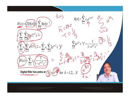
Now, what is H(z)? So, suppose h[n] is my impulse response, then H(z) is equal to the Z transform of h[n]. What is the Z transform?  $H(z) = \mathcal{Z}\{h[n]\} = \sum_{n=0}^{\infty} h[n]z^{-n}$ . Now, I know h[n] is this one because this is the continuous impulse response, the continuous time I sampled the T into n into T, so this is my h[n], so I put this h[n] value is in here ok.
