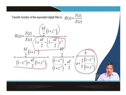
So, I get H(z), just then, the just simplification bT by 2 a 1 plus  $z^{-1}$  into aT by 2 so, all aT will be  $z^{-1}$  will be there and so, all if I make that simplify it, it will come in this form b by a plus 2 into 1 minus  $z^{-1}$  divided by 1 plus  $z^{-1}$ .
