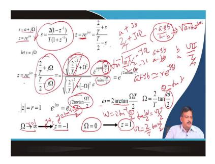
And then mapping, then else is what? The mapping between s-plane and z-plane. So, s is equal to a plus j  $\omega$ , z is equal to  $re^{j\omega}$  so, s is equal to this one I know. So, I can say z is equal to  $re^{j\omega}$ . So, what is z? z is nothing but a 2 by T plus s divided by 2 by T minus s. So, r  $e^{j\omega}$ , which is nothing but a T by 2 plus s T by 2 minus s.
