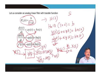
Let us say I have an H s a b by s plus a, so I have to convert H(z) using bilinear transform, a trapezoidal formula I will come to that. So, if I say that H of a s is equal to so, I can say H of a s into s plus a is equal to b. So, now, if you see, if I have a system which has an H, s is my transfer function, if I apply X(s), I get Y(s), so Y(s) divided by X(s) is equal to
