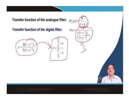
So, what I have taken as an H s? So, H s is equal to b by s plus a. H(z) is equal to b by this plus a. So, I can say this is nothing but a s, if this is s, then I can from this equation, I can calculate what is z ok.
