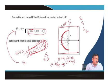
Then what is the relationship? How do I design the transfer functions? So, for a given order of the filter, I know the pole position. Now, pole position sk I know. So, what I know, I know s0, I know s1, I know s2. Now, if the filter wants to be a stable filter and causal filter, then all the poles must be located in the left-hand plane of the s plane, which is the s plane.
