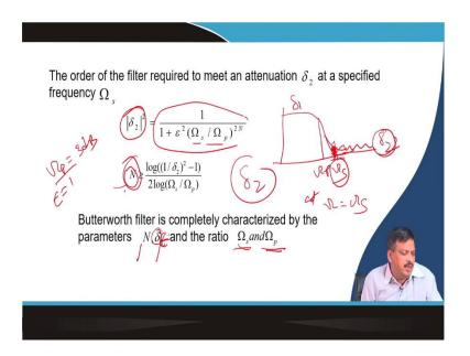
Now, I come. The order of the filter is required. So, how do I define the order of the filter? How do I define the order of the filter from the given specification? So, what is given in the specification? It gives passband edge frequency  $\Omega p$ , given stopband edge frequency  $\Omega s$ , given stop band ripple.
