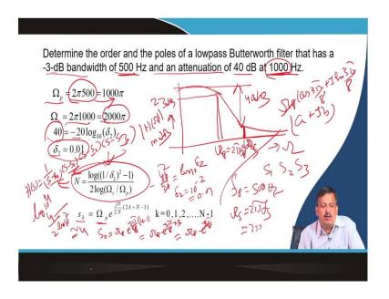
So, let us get it. I think there is an example. Let us take an example. I said to determine the order and pole of a low-pass Butterworth filter that has a minus 3 dB bandwidth at 500 hertz and an attenuation of 40 dB at 1 kilohertz. So, what is it? First, you draw the picture. So, I can say there is a pass band at 3 dB; Butterworth, let us say this kind of thing, at 3 dB down, let us say this is 3 dB down.
