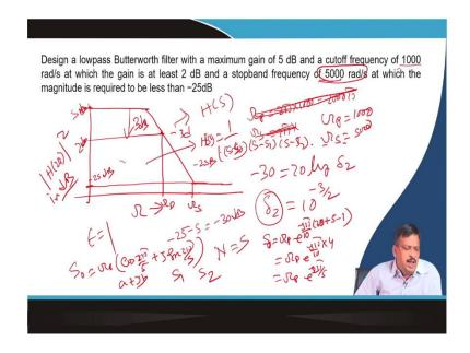
So, what is the example? Design a low pass Butterworth filter with a maximum gain of 5 dB and a cut-off frequency of 1000 radion at which the gain is 2 dB. So, let us first draw the frequency response of the filter. This axis is the  $\Omega$ , and this axis is the mod of  $H(\Omega)$  whole<sup>2</sup> in dB ok. So, I what I said? I said this is 5 dB, gain of 5 dB, then it is decreased to 2 dB. So, it is here it is 2 dB, so this is 5 dB. So, how much is decreased? This decreases by 3 dB.
