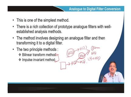
If you look at the analogue filter, this method is the simplest method because analogue filter design methods were available long before the digital filter came out. So, design methods for the analogue filters are always established. So, there are a lot of prototypes for designing analogue filters: Chebyshev, Butterworth, and elliptical. So, all kinds of prototype filter design methods are available and have already proven to be very good methods.
