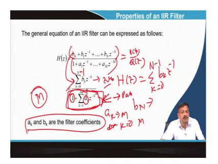
So, how do I design how what should be the expression of an IIR filter? What is a general solution for an IIR filter? So, I know IIR filter H(z) is nothing but a P(z) by Q(z). So, it is nothing but a 2 polynomial, one up and one down. So, this polynomial can be written this way: also, k is equal to 0 to n bk  $z^{-k}$ . Ok or not? If it is an FIR filter, this feedback is absent.
