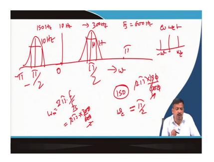
Whose centred frequency is 150 hertz, the bandwidth is 10 hertz, and the signal maximum frequency is 300 hertz. The sampling frequency F s is equal to 600 hertz. So, if I want to draw the magnitude spectra. So, let us see this is my 0, and this axis is in  $\omega$ . So, I know what the highest rate of oscillation is in the case of a digital signal. It is nothing but a  $2\pi$  into f by F s  $\omega$  s  $\omega$  m.
