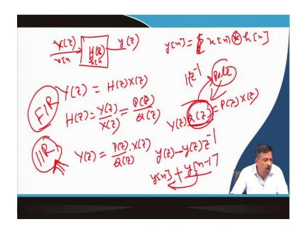
I have a system called H(z). If I apply an input X(z), I get output Y(z). Now I know Y(z) is equal to H(z) multiplied by X(z) or if it is h[n] if it is x[n], then I know y[n] is equal to the convolution of x[n]; x[n] convolved with h[n] that I know. Now, what is the H(z)? I can say H(z) is nothing but a Y(z) divided by X(z).
