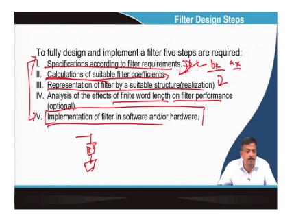
So, if you summarize that filter design step for the IIR filter, that is a five-step—specification according to the filter requirement. So, I have to require a filter specification, let us say design and IIR filter low pass IIR filter cut off frequency 2-kilo hertz transition bandwidth this refill this.
