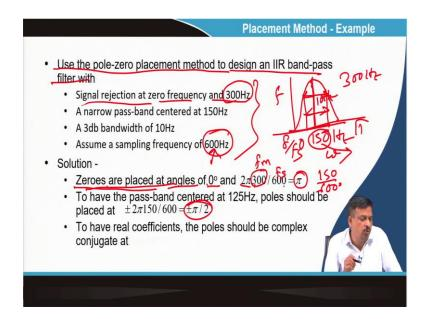
Let us say direct methods. This will be an example of the direct methods. So, what is the direct method? Use the pole-zero placement method to design an IIR band pass filter. Let us say this: I have to design. So, what I said is that I have to design and bandpass filter narrow pass band centre at. So, 150 hertz is the centered frequency, and the 3dB bandwidth is 3dB bandwidth is 10 hertz.
