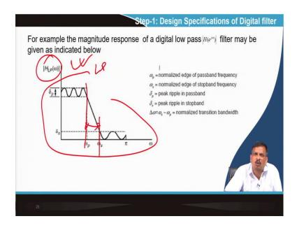
So, the first step is the design specification, the same as the FIR filter. So, this is nothing but the magnitude response of the low pass filter, which is a pass frequency, stop bandage frequency, transition bandwidth, ripple in the pass band, and ripple in the stop band.
