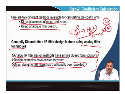
So, all are the same requirements here. The next step is a calculation of the coefficient. How do I derive ak and b k? That is my target. There are two different methods available for calculating the coefficient. One is called the direct placement of pole and zero; one is called using the analogue filter method. So, there are two methods available to compute ak and bk. One is called direct placement; another is called using analogue filtered design methods.
