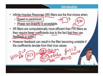
Now, why IIR filter? You may say that, sir, I know the FIR filter and the design is very simple, so why should I use the IIR filter? Now you know that the IIR filter is computationally more efficient than the FIR filter, which I have already discussed. Because the IIR filter required fewer coefficients due to the use of feedback or poles, I will describe it in detail.
