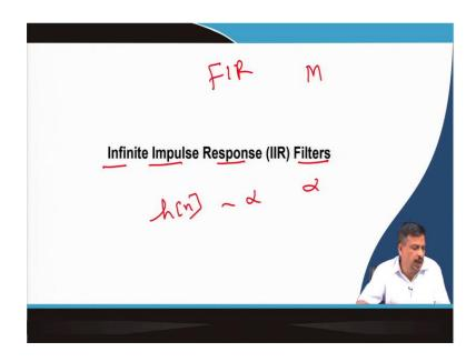
So, we have talked about the FIR filter and finite impulse response filter. So, FIR, where M is the finite order of the filter, is finite. Here, I am talking about the infinite impulse response filter. So, where I have an h[n] whose length is infinite, it is from minus infinity to infinity. So, an infinite length filter is an impulse response length filter. So, that is called an IIR filter, ok.
