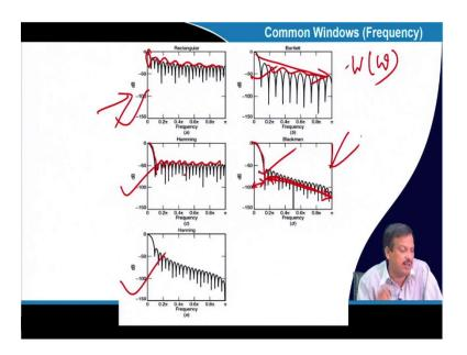
And every window function has its own frequency response. So, those are nothing but a  $W[\omega]$ . So, we collect some samples of, let us, 300 samples of the windows using this function. How do you do the frequency response? Let us see this Blackman window.
