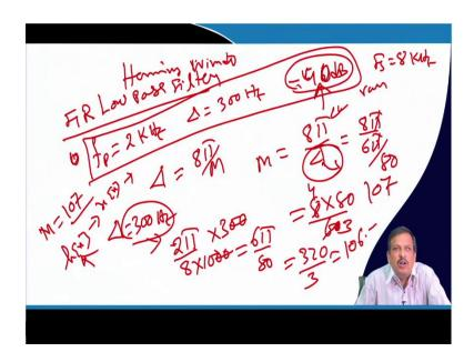
So, I want to design a filter using a Hamming window. So, what is the if you see when I say the Hamming window, I know the peak side lobe is minus 43 dB. So, if I require a very much attenuation in the side lobe, then I can go for a Blackman window minus 58
