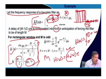
So, let us say this is my low-pass filter frequency response. What is required? Up to  $\omega$  c up to  $\omega$  c, this is 1, amplitude is 1; else, it is 0. This is my requirement;  $\omega$  c is the cut-off frequency. Now, a delay M minus 1 by 2; so, M is the order, and M is the order of the filter M minus 1 by 2. So, M minus 1 by 2 unit is incorporated into H[ $\omega$ ]. So, why is this term incorporated? What is required?
