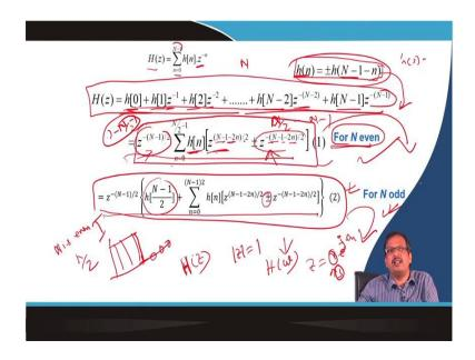
So, how do I design what should what kind of frequency response we will get if I design a linear phase filter? So, what is H(z)
