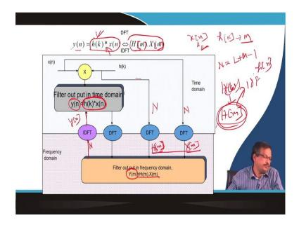
Now, if you see another view, let us know if this can be implemented in the frequency domain. So, as I know, the frequency y[n] is a convolution in the time domain. So, in the frequency domain, it is nothing but the multiplication ok or not? In the time domain, it is convolution. So, the frequency domain is multiplication.
