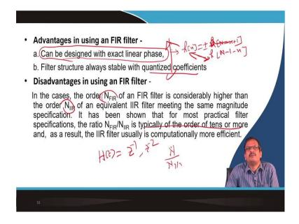
Now, I come to the advantage. Why are we talking about the FIR filter most of the time? Many times, we have not talked about the implementation of IIR filters in digital filters.
