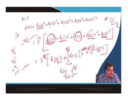
So, now I said N is odd, let us take a small example: N is equal to 5, and N is odd. So, I can say H(z) is equal to h[0]  $z^{-0}$  plus h[1]  $z^{-1}$  plus h(2)  $z^{-2}$  plus h(3)  $z^{-3}$  plus h(4)  $z^{-4}$ . So, h(2) 3 4 5 order is mentioned 5 order n is equal to 5.
