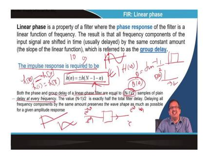
Now, we come to the linear phase. What is a linear phase? I am not reading the slide. You can read it. So, linear phase is a property of a filter where the phase response of the filter is a linear function of frequency. So, you know the magnitude response  $H[\omega]$  mod of  $H[\omega]$  magnitude response and tan inverse, you know that tan inverse imaginary part divided by real part is the  $\theta$ .
