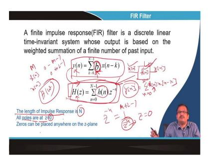
So, as I said, the FIR filter is nothing but a finite impulse response filter. So, this b k, I can say, is nothing but a filter coefficient that is represented by h[n] understand or not. So, this is the H(z). So, what is the output? Output is the filter coefficient. So, if I say a filter is a system, this is h[n], let us say this is x[n]. So, the output is y[n]. So, when I say what is y[n]? It is nothing but a convolution between x[n] and h[n].
