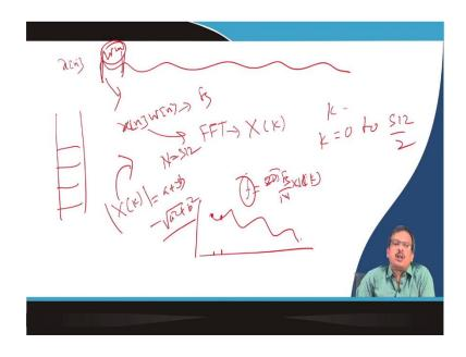
x[n] is given, which is non-stationary. So, I have a long signal, and I select a portion I want to the spectra.
