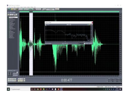
So, suppose I want to know what the spectrum representation of this portion of the signal is. So, once I select the portion, I will be doing a short Fourier transform.
