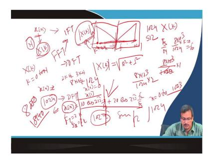
So, I have a signal x[n], and I want to draw the signal's spectrum. So, what is spectrum? The spectrum of the signal is nothing, but when I plot this axis, it will be the frequency, and this axis will be the amplitude of individual components. So, let us convert x[n] to X(k) using the FFT algorithm.
