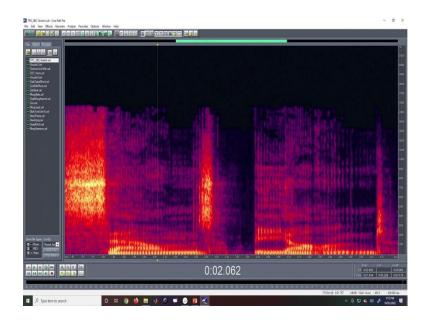
So, more yellow means more power, and more prominent in the frequency means that frequency has a higher power. If you look at, I think this axis in the spectrogram this axis represents this axis represents the frequency, this axis represents the frequency, and this axis represents the time.
