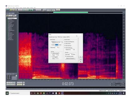
Window function, which window function, what resolution, how many bands you required, window width 70 plus overlap. So, all kinds of settings you can do. So, suppose I told you to write a program for computing a spectrogram or representing the spectrogram of a signal.
