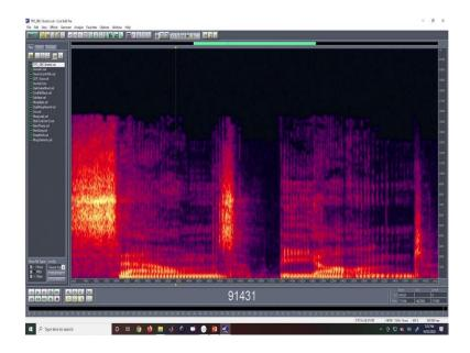
Suppose these cases are in this demo case; how many samples are there? In the signal, if I click it here, it comes to the samples 142368 samples are there. So, if I compute a spectrograph and want to draw the spectrogram by sample by sample, it takes a huge
