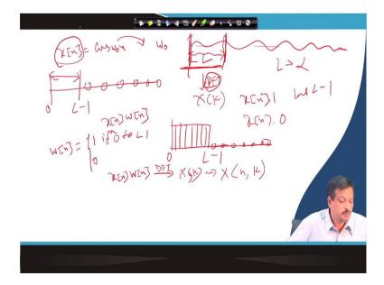
I am saying I have a signal x[n], which is, let us say,  $\cos(\omega 0n)$ . So, the frequency of the signal is  $\omega 0$ , and that is  $\cos(\omega 0n)$  has a long sequence; let us L tends to be an infinitely long sequence. So, I cannot take the whole sequence to analyze discrete Fourier transform at a time.
