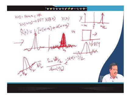
So, when I say my signal is only  $\cos \omega x[n]$  is equal to  $\cos(\omega 0n)$ , then what is the frequency transform? What is the frequency representation of a cos function? If this scale is frequency, this is 0; then I said there would be one component in here, which is  $\omega 0$  plus, and one component will be here, which is  $\omega 0$  minus.
