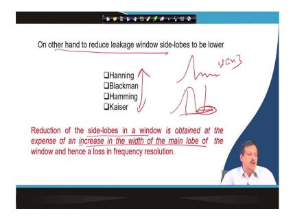
Now, if you see that window requirement, how do I define it? So, that side lobe produces a leakage. So, if I want to reduce the leakage, there are different kinds of windows: Hamming window, Hanning window, Blackman window, and Kaiser window, which reduce the side lobe at the expense of increasing the width of the main lobe.
