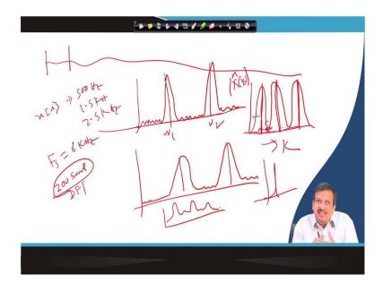
So, in summary, when I want to analyze a signal in the frequency domain of a long signal, I have to multiply the signal within the window. And the choice of the window depends on what I want. If I say I use a rectangular window, the leakage is much greater. So, if I
