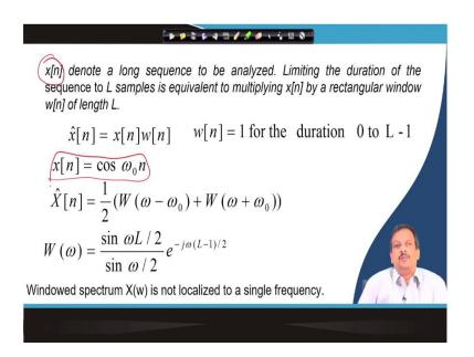
Let us say in the case of a x[n] is a sequence long sequence of a signal that has to be analyzed, and let us say x[n] is nothing but a  $\cos(\omega 0n)$ . So, I have a signal that is nothing but a x[n], which is  $\cos(\omega 0n)$ . So, what am I saying?
