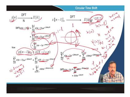
Similarly, if I go to the circular time shift, another property is circular time shift. x[n] is my signal, and DFT is capital X k. Now, if I say circular time shift because I know x[n], if the N point DFT is calculated, then the period is N and x[n] is repeated circularly. So, x[n] is repeated circularly with N. So, I have to make a circular time shift. So, I have to shift within. So, I can say, as you saw when you do the circular time shift, what do you know?
