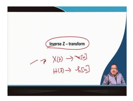
Ok. So, in the last class, we discussed about the pole-zero concept in the Z transform. Now, in this class, we will try to discuss the Inverse Z transform and what an inverse Z transform is. So, if you see the inverse, what do you mean by that? So, I have an X(z). Can I get back x[n]? So, X(z) is given to me, I want to find out the x[n] like the H(z) is given to me. The transfer function is given, and I have to find out the impulse response of the transfer function.
