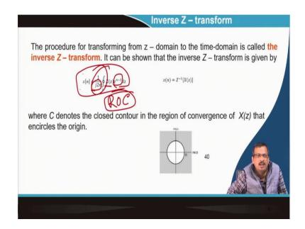
So, that is called inverse Z transform. What is its definition? The procedure for transforming from the Z domain to the time domain is called inverse Z transform. So, X(z) is given, I have to convert to time domain signal x[n].
