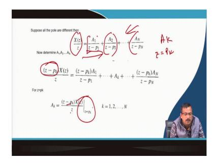
Now, I said I suppose this X(z) by z that can be a summation of A1 by z to the power z minus p1 A2 by  $z^{-p}$  that can be. So, I can factorize the lower portion, and I can express it in terms of this summation. Now I have to determine A1 A2, and An how do I determine A1 A2?
