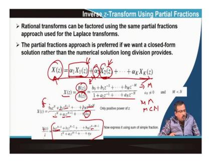
The next one is using partial fractions. So, rational transformation can be, you know that I am not reading the slide. You can read on the slide. So, what is what I do with partial fraction, what do you mean by that; that means, suppose I have a transfer function I have a transfer function X(z) somehow, I have to break it so that it consists of, let us say X1(z), X2(z), Xk(z) because the superposition principle is support this document linearity is supported.
