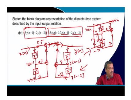
So, let us start with some problems. Sketch the block diagram representation of the discrete-time system described by the input-output relation. So, this is the input-output relationship.
