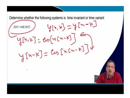
Another problem is determining whether the following system is a time-variant or time-invariant, time-invariant or time variant. y[n] equal to  $\cos of x[n]$ . What is the procedure? The procedure is that y[n,k] must be equal to y[n-k]. So, let us say k time after k time, what should be the so, I know
