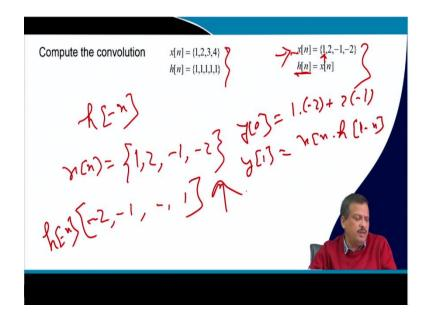
Compute the convolution. I have given two problems; this is one problem, and this is another problem: compute the convolution. So, if I do this one convolution. So, what is the formula for convolution? So, I know x[n] and h[n] must be the same. So, I can once I folded. So, h[n] I have to calculate h[-n] I folding it. So, if I have a x[n] this one 1, 2 let us say this one is the 0th sample; minus 1 minus 2 then if I fold it that means, reverse so, minus 2 minus 1, 2 then 1 h[-n].
