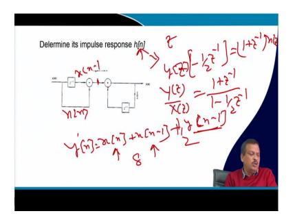
Determine the impulse response of h n I have given. So, what is the impulse response? I can say this is x[n], this is x[n-1], and this is x[n]. So, I can say this point is x[n] x[n] plus x[n-1] plus y[n-1] multiplied by half is equal to y[n]. Now, if I say that z to the power if we want to find out the h[n] in impulse response in terms of z domain or impulse response.
