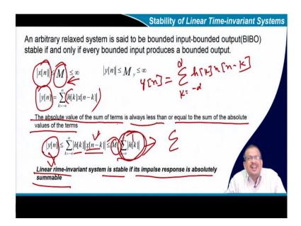
Now, I come to the stability of a linear LTI system. How do I calculate the stability of an LTI system? So, what is the definition of stability? I have already discussed this in this week's lecture. What is the definition? The definition is that if I apply a bounded input, the output must be bounded, and then I can say the system is stable.
