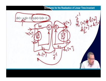
Then, the realization of the LTI system. This is very important. Suppose I have this system; how can I realize this system using a computer? How do I realize this system? So, I know this is y[n], ok, and this is x[n]. So, if you see that the x[n] will be multiplied by b0 and the one sample delay  $z^{-1}$ , x[n-1] will be multiplied by b1 and added up. So, I get up to this. This part I have done.
