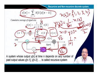
Now, there is a recursive and non-recursive discrete system. We have already learned about the recursive algorithm and recursive system. So, what are recursive and non-recursive discrete systems? So, I have an h[n], which is the output of a system, convolution sum. So, a cumulative average of a signal; suppose I have a signal x[n]. I want to calculate the cumulative average.
