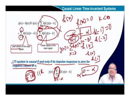
Now, we will discuss some linear time in variant systems, like causal, stability, etc. So, I said causal linear time-invariant system. So, how do I write the expression of the convolution? So, as you know, what is the convolution? k equal to minus infinity to minus infinity to infinity.
