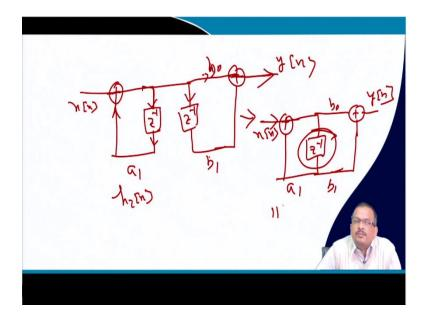
So, I have an x[n], and I will interchange  $z^{-1}$  and a1 and add up. So, this is my h2[n], plus this is my y[n]. What do I do?  $h^{-1}$ . This is nothing but a b0; this is nothing but a b1 and added up. So, this portion I have used in here and this portion I have used in here, so I interchange. So, I get this one.
