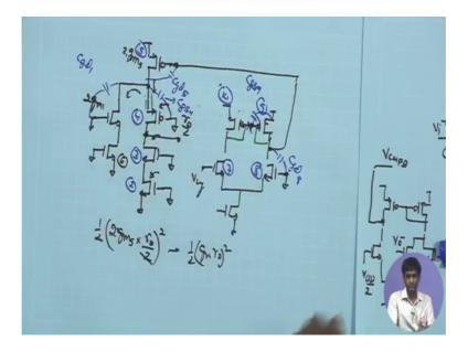
So, this is going to be 2 times gm one because after clubbing these 2 common mode we had W by L getting twice and I getting twice therefore, 2 times gm one and gate is anyway AC ground and you have the you call this six. So, you have the m 6 also the gate being AC ground.
