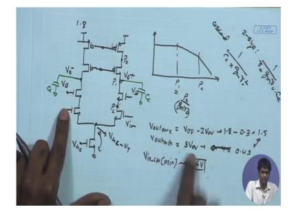
Then it was you know violating my minimum allowed same voltage level over here which was point 6 volt, but here that is on the case I can allow I can have a input DC point which is not conflicting with my output common mode level.
