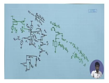
So the basic operation involved in the folded cascoded is you can start with the ideal current source, where our input device is the NMOS and you are having the cascode operation being provided by PMOS device and then you have another NMOS load. This is a single ended cascode we were looking into the differential version of that also. But it is important to look at the functionality here once we are comfortable with this we can go for a differential version.
