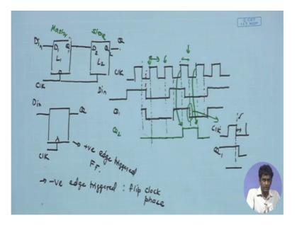
Let us call it D 1 Q 1 D 2 Q 2. And you have the output of Q 1 connected to the input of the second latch. So, I can call this latch 1, L 1 let us call this latch to latch 1 is low level sensitive. So, this becomes transparent when the clock is low, that is denoted by this bubble. And we have the latch 2 which is high level sensitive.
