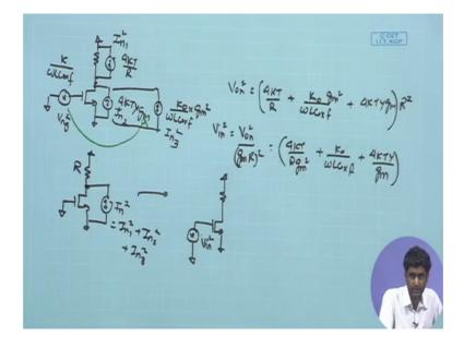
So, we can start the analysis with a simple common source amplifier with resistive load and then go towards active load amplifier which is ultimately going to link with our overall two stage amplifier with the help of which we have been building our fronted amplifier. So, here I have considered a simple common source amplifier and I can represent the overall noise constituent of these two resistors and the transistor over here.
