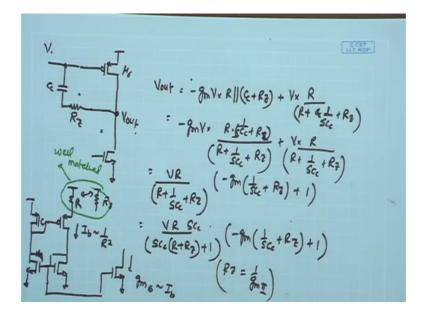
And that basically involves insertion of a nulling register in series with the cc. So, once again I have the second stage, I have just inserted another nulling register Rz in series with cc and therefore, I once again need to analyze the expression for v out in terms of the v in over here, and to do that once again we will revisit my previous analysis where I had used two parallel paths and arrived at the expression for the output in terms of the viewing.
