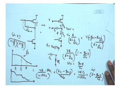
So, here if I look at the second stage, you are having the C c between the input of the second stage and output for compensation and result we have 2 different signals paths one coming from the input to the output through the C c and another one coming from the drain of the MOSFET. So, if I for example, if I isolate these 2 if I isolate these 2 resume these are 2 independent signals being applied at the input of the second stage.
