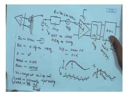
So, in our earlier specifications; we have not discussed two very important characteristics of differential front ends that is the common mode rejection ratio and power supply rejection ratio.
