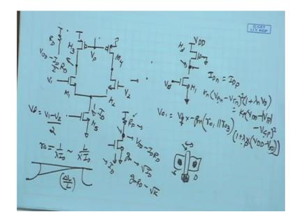
Let us get started with simple fully differential amplifier using MOSFET transistors. This is a single stage fully differential amplifier provided you have a bias point to V p you call this M 1, M 2, M 3, M 4, and M 5 and we are assuming that V p had been provided by appropriate biasing scheme and we will be discussing that very soon.
