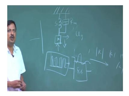
So, what is the what is the form of a mechanical oscillator? There is a spring there is a mass and there is a mechanical damping. This is the mass this is the spring constant s and this is the mechanical damping R m ok.
