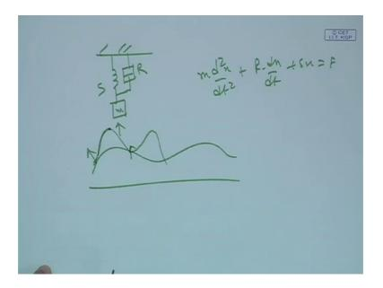
If you remember that spring mass movement of a body mechanical vibration spring mass movement if you remember that m S and R. So, you know that d 2 m into d 2 x by d T square plus r into d x d T plus S x is equal to force the force which is applied.
