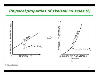
So, d T by d x is equal to b into T plus a T is a tension b and a are constant.
