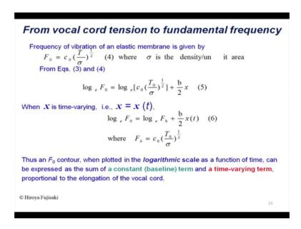
Now if it is T 0 e to the power b x, then frequency of vibration of elastic membrane F 0 is depends on C 0 into T by sigma to the power half where sigma is the density per unit area unit area density per unit area this is relationship between the elastic membrane vibration membrane vibrations.
