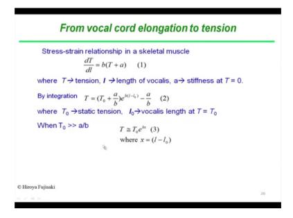
Now if a by b is much much less than T 0 then I can say T is equal to T 0 e to the power b x T 0 e to the power b x which is there in here which is equation 3.
