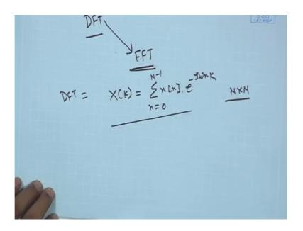
So, FFT is not the transform. FFT is an algorithm to implement DFT. That is why it is called fast Fourier transform algorithm, fast Fourier transform FFT. So, FFT is an implementation procedure for DFT. So, if I say that DFT is nothing but a x of k is nothing but a sum of n equal to 0 to n minus 1 x of n into e to the power minus j omega n k. So, how many number of complex multiplication is in here n cross n? N cross n complex multiplication is there.
