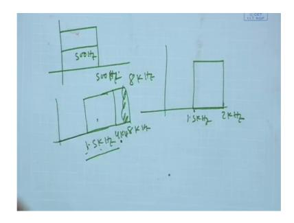
Now, I want to implement a band pass filter of 500 hertz bandwidth with a frequency between the 1.5 kilo hertz to 2 kilo hertz. So, what I will do? I will just shift this low pass filter to 1.5 kilo hertz frequency. So, that I get this one understand or not.
