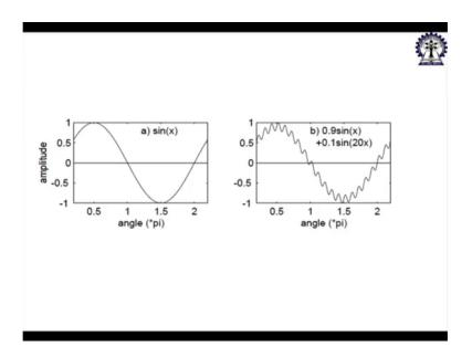
So, in that case I fail to detect the f 0. So, 0 crossing rate base f 0 detection is not Very good solution or good methodology for finding out the f 0.
