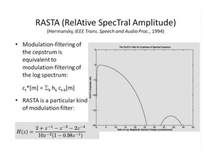
So, RASTA also there is a 1 another side. So, it is a modulate, relative spectral amplitude modulation filter of spectrum is equivalent to modulation filter of log spectrum.
