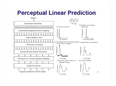
So, what is said take the speech signal find out the first Fourier transform then calculate the cepstrum. And modify the cepstrum as per the critical brand or Mel frequency cepstral cepstrum or bark scale, then modify the equal the modify the loudness. Loudness of the amplitude of the cepstrum as per the equal loudness curve. Then apply the power law of hearing what is power law. If you remember that relations between the loudness and intensity, I think it is 4 4 5 into I to the power 0.333.
