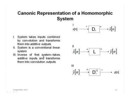
So, if you see this picture, there is a three 1, 2, 3 - three part. First part system take input combine by convolution and transform them into additive output. Second part system is conventional linear system I can suppose linear filter inverse if first system take the
