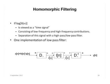
Then you can discuss the homomorphic filtering. So, if log x omega then I can pass through a. So, in view of the time signal, I can pass the low pass filter and I can find out the slowly varying component. So, I can say I am not going details of that in the filtering technique of here.
