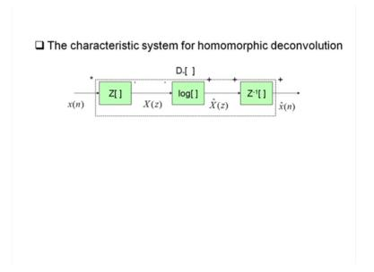
So, if I want that I want that convolution should be represented in a some form, then the system transform function should be like this.
