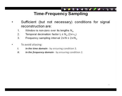
So, now I take a example so, window length is N w, take window length is N w, so temporal decimation factor L must be equal to n w less than n w and L must be equal to 2 pi by omega c and 2 pi by N must be greater than 2 pi by N w.
