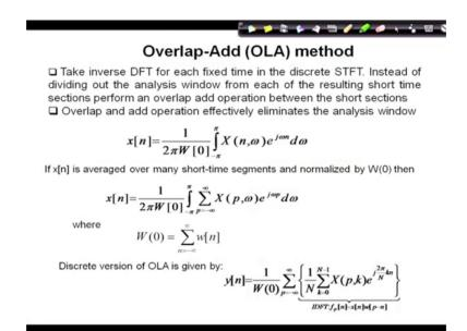
Another method of be since in synthesis is that, overlap add method, so this is another method of STFT synthesis this is call overlap add method. So, in overlap add method, so take inverse DFT for each fixed time of the discrete STFT instead of dividing out the analysis window from each of the resulting short time section I can do a add operation.
