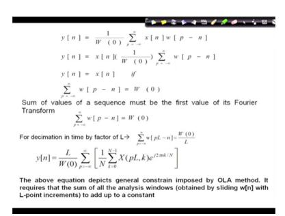
So, I can say next y n what is the y n in overlap add method y n is equal to 1 by W 0 into p equal to minus infinity to infinity so, all segments I sum up x of n into w p minus n. So, I can say it is nothing but a x of n divided by W 0 into p of minus infinity to infinity w p minus n.
