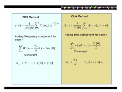
So, if I summarize FBS method the constant is this 1, which define me the size length of the analysis window must be less than the number of analysis channel, and OLA method define a constant which omega c the bandwidth of the analysis window must be less than 2 pi by N 2 ok.
