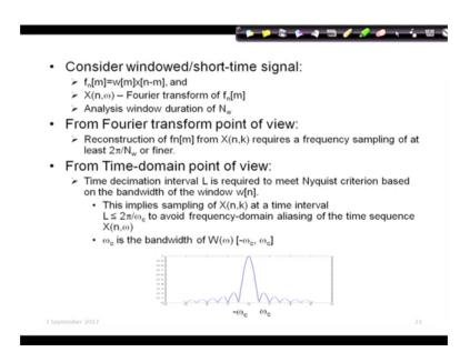
So, considering window for time signal f n omega is equal to omega w n into x n and x of n omega Fourier transform of x n analysis window is n w, so Fourier transform point of view reconstruction of f n omega f n m from x n k require the frequency sampling at least 2 pi by N w.
