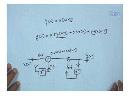
So, discrete system; let us output of a discrete system is y n is nothing, but a H of input x n. So, H is the transfer function of the systems lets the system is like this y n is equal to 0.8 y n minus 1 plus 0.5 x n plus 0.9 x n minus 1.
