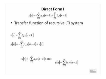
You can practice it; now implementation is important. So, how do we implement a discrete system there is a 2 kinds of implementation one is called direct from one and one is called direct from 2. So, one is called structure one implementation another is called structure 2 implementation.
