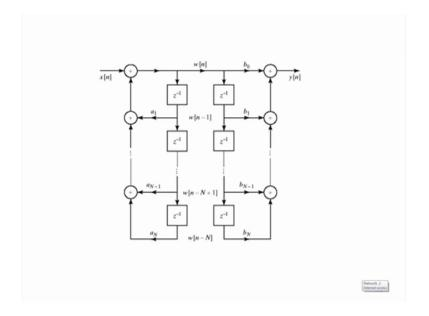
This is I said that I long this is one block and this is block once to interchange it will come same side. So, instead of 2 Z to the power delay I can club together and put the single delay. So, it is called delay from 2 implementation.
