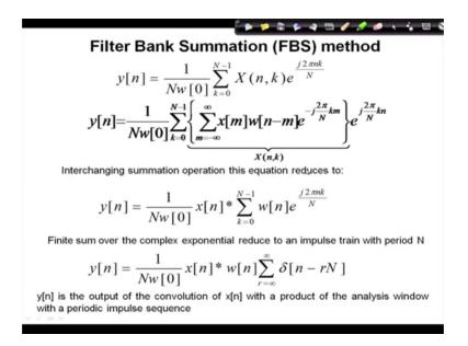
Now, if I interchange the summation operation this equation this equation reduce to one by nw 0 x of n convolution with k equal to 0 to n minus 1 w n e to the power j 2 pi by nk. So, I can write after putting value I can write w yn is equal to 1 by N w 0 ok.
