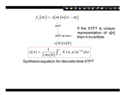
Which is nothing, but a xm multiply by the window function I take the DFT and then I take the IDFT and evaluated at m equal n I get x m multiply by omega 0. So, xn is nothing, but a inverse Fourier transform of frequency domain representation of STFT with 1 by 2 pi into w 0. So, this is a synthesis equation of STFT analysis, now what is the
