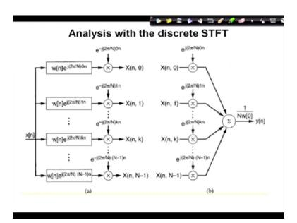
What we done we pass the signal through the window then we modulate the signal or you can say demodulate the signal or shifted the signal e to the power minus j 2 pi by N by 0. So, that is this is the synthesis equation this is the synthesis block portion, now if I
