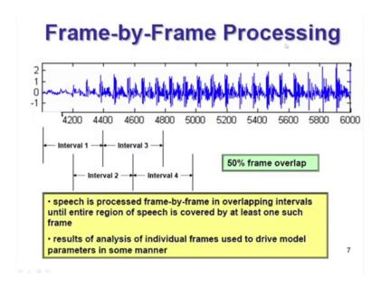
So, this is the example if it is it is here, so this is the interval 1 and then, shifting of the frame by 10 millisecond or less 50 percent, if it is 20 millisecond window 50 percent of overlap means 10 milliseconds Shifting.
