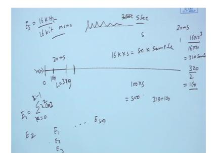
So, put the microphone connect to the computer record your name, once you let your name consists of three second signal all let us 5 second signal long name 5 second signal it is consist of 5 second speech signal so; that means, 16 kilo hertz sample 16 k sample per second, so I can get 16 k into 5 80 k sample ok.
