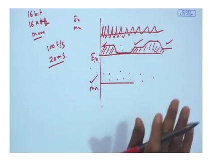
So, if it is short term energy then, I can find out let us this is my signal x n whose sampling frequency is F s I operator is x of so, I can say square; square, is the operator signal square I take the signal square then, I pass the signal, so all signal is every sample is square rate is still F s. Now once I pass through the window W n after the window my
