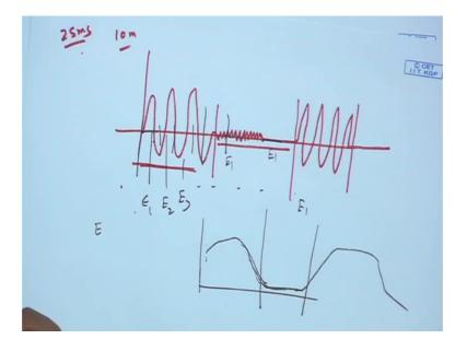
So, I get 100 frame per second, I can take 25 millisecond as a window and shift at the frame 10 millisecond that also I get 100 frames per second ok.
