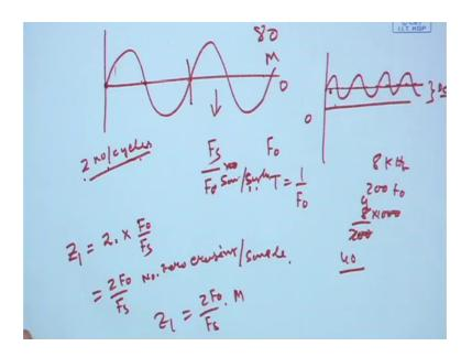
So, how many time signal crosses the 0 line, so it is 1 2 if it is period, so if it is I start from 1 then 1 2 then this point is part of the next period. So, I can say if it is a pure sine wave then 2 number of zero crossing per cycle; per cycles, 2 number of zero crossing ok.
