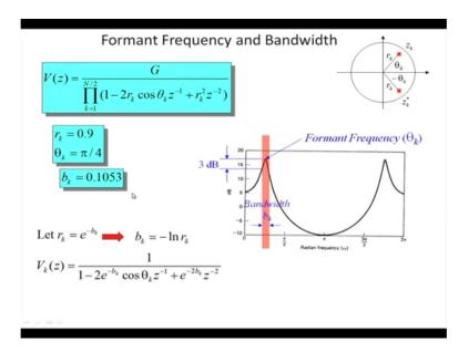
And theta k give the formant position. When the value of r K approach to unit I can get the formant frequency resonance frequency. So, if it is r K approach to unit circles to unit circle then I can get the resonant frequency. And if the bk right bk value is non 0 then I get a band width pole, there will be a pole there will be a formant which has a band width. So, bk provide me the band width theta k provide me the formant position.
