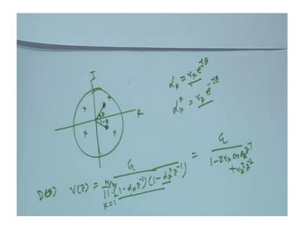
So, complex conjugate pole. So, this is the real axis this is the imaginary axis. If a pole occur in here with a angle of theta. There will be a another pole which is conjugate this pole minus theta and here. So, if there is a pole in here there is a another pole will be in here, if the pole in here there is another pole will be here.
