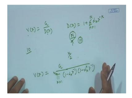
So, I can say the vz is model using G by dz where dz is equal to 1 plus k equal to 1 to N alpha k z to the power minus k. So, dz has an N if it is order is n. So, N number of pole. So, I can say vz is a all pole model which has N number of pole. So, if I have a 10 junction tube 10 tube 10 10 section tube then I can say 10 poles will be there 10 poles will be there. So now, if dz is real. So, the dz have either the all re real pole will be the real functions.
