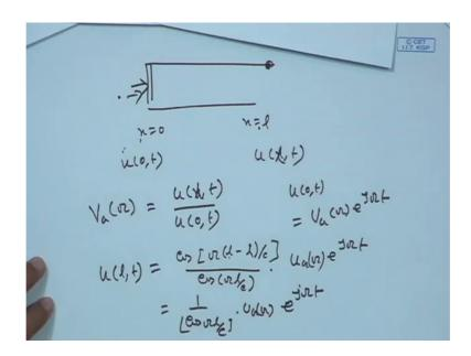
So, if I say input is u 0 t and output is u x t volume velocity. So, I can say the v a transfer function v a omega is nothing but a u x sorry u 1 t u 1 t divided by u 0 t. X is 1 and x is 0 here. So, what is that?
