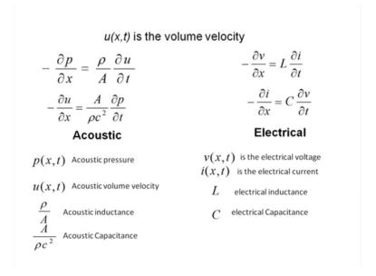
This is del u by del t, not del p, del u by del t is or rho c square by a del v by del x. Or I can say del u by del x is equal to minus A by rho c square del p by del t.
