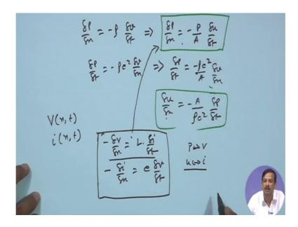
Where I can say that del square or del p by del x is equal to minus rho del v by del t. So, this will become v is equal to u by A. So, del p by del x is equal to minus rho p u by A, rho by A del u by del t. Similarly del p by del t is equal to minus rho c square, del v by del x this will become del p by del t is equal to minus rho c square, rho c square minus rho c square, or I can say del u sorry.
