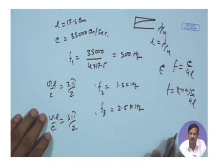
So, I is equal to 17.5 centimeters what is c? Velocity of sound velocity of sound is 3 5 centimeter per second.
