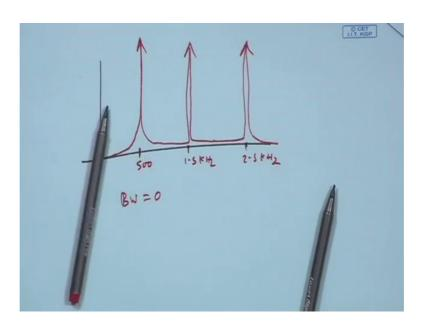
So, it is I can put an arrow in here. So, it is infinite power; infinite impulse with the impulse power at 500 hertz, and bandwidth is equal to 0. This is a real pole. So, bandwidth is equal to 0. Bandwidth is equal to 0 with 0 bandwidth, infinite power resonance will occur at 500 hertz, 1.5 kilo hertz, 2.5 kilo hertz, if the length of the vocal tube is 17.5 centimeter and velocity of the sound is 35000 centimeter per second.
