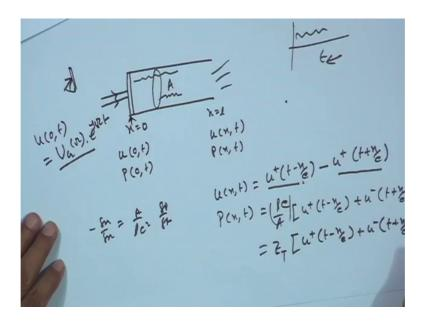
Which is I can say this side is the vocal cords which acts as a piston. And so, x is equal to 0 where the force is applied in the tube and x is equal to 1 where the tube radiate the sound energy in the air.
