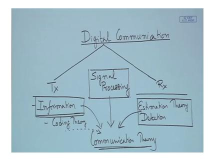
Now, coming back to the issue which I was trying to bring out to you. So, if we look at digital communications, we can broadly divide it into 2 sides one is the transmitter side, the other is the receiver side. In every where you will find we are essentially doing signal processing right. All the things that we did at the receiver channel estimation equalization carrier frequency estimation clock estimation are signal processing.
