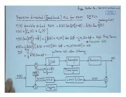
So, we will take a look at the decision feedback or decision directed PLL for pulse amplitude modulated signals. So, it is called d f PLL and in this case the received signal r t is a double side band signal. So, the PAM is A t cos 2 pi f c t and at is a m g t. So, that is how we have this particular signal.
