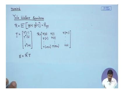
The next set of interesting relationships which matches our requirement are the; we Inerhopf equations for linear transversal filter. So, that says from orthogonally principle the input must be orthogonal to the errors we will see more of it, right. So, that the weights that we choose ensure that the inputs are orthogonal to the error; that means, the inner product would produce a 0.
