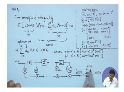
So it assumes that the input goes through linear transversal filter coefficients, we have to find. So, there again the coefficients can be formed using these relationships. So, they all give us the same kind of result which we can exploit in finding filters which will produce the desired response; that means, it will produce an error which is minimum in some sense.
