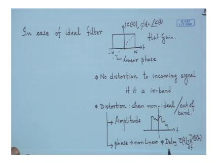
So, in case of an ideal filter; so let us start with the ideal filter because that is the simplest thing that we can begin with. So, here the channel amplitude is flat over the desired frequency that is W and we have stated previously that beyond W; it is 0. So, the channel; not the pulse, the channel is said to be 1 which is ideal; that means, no amplitude distortion and there is linearity of phase.
