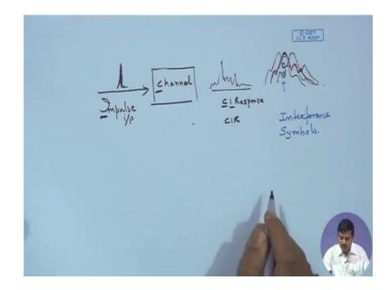
So, when we talk about the channel impulse response; so, the channel impulse response is defined as the response of the channel, when an impulse is launched into it. So, one can think of the channel as a system or as a filter as we said and if you launch an impulse into this; if I am going to launch an impulse into the channel whatever is the response I am going to get out of the channel would be the channel impulse response. So, channel impulse response and that is known as the C I R.
