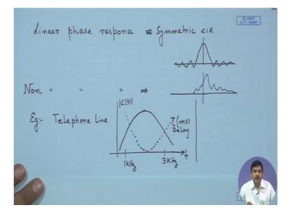
So, the linear phase response as we just mentioned results in a symmetric channel in pulse response. We will quickly see what is meant by the channel impulse response; however, if the phase is non-linear, the impulse response would be asymmetric and it could take; for example, a situation which is like this.
