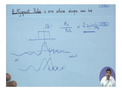
And the maximum possible symbol packing rate, 2 W symbols per second over a bandwidth of W or you can think of R S symbols per second over a bandwidth of R S by 2, it results in the same thing. You have R S symbols per second over bandwidth of r s by
