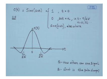
So, moving ahead c of t as we have written here is sinc, so sinc as you know has a 1 at t equals to 0 and 0 at all other sampling instance; at all other locations where 2 W t equals to n; this is well known. And elsewhere it follows the sinc function, so if you plot it; this looks over here because we have a 2 W; it turns out to be 1 by 2 W.
