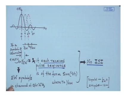
So, if we are launching signals every T duration; so, if we launching a T, 2 T, 3 T such that T is equal to 1 by 2 W, what we find at sampling instance; all other echoes go to 0. So, that clearly means that we can launch signals at every 1 by 2 W seconds.
