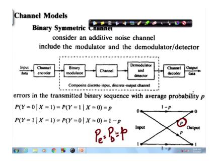
And these are clearly due to the noise effect, which you can easily see that because of noise you have a certain probability of error. So, probability of error in this case; it is probability of bit error which is equal to p. So, here the noise is getting translate to a transition probability.
