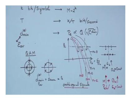
So, looking back at some of the schemes that we have studied; we could say that we have looked at situations where k; which is the bits per symbol is one of the important factors which is used to choose the constellation size; which is M is equal to 2 to the power of k, so, as k increases we have seen that M increases.
