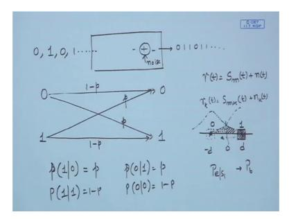
So, we construct the channel out of that; it goes through the channel passes through AWGN and demodulator detector and again it produces a sequence of 0's and 1's.
