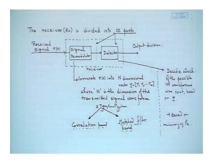
And then we looked at the receiver architecture where we said that the received signal is first demodulated. So, it goes through a demodulator and then it goes through the detector you have typically studied demodulator in analog communications and you will see some form of similarity in this as well.
