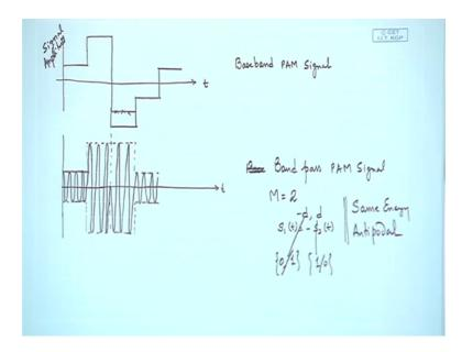
And we would just try to complete our earlier discussion on PAM by trying to see the waveform in the pass band and base band with given a rough picture earlier we will try to give a clearer picture this time.
