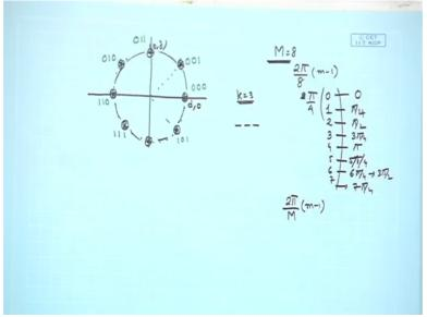
So, you are going to get 2 pi by 8 multiplied by m minus 1 or you are going to get pi by 4 multiplied by 0 1 2 3 4 5 6 and 7 that is what you are going to get leading to 0 leading to pi by 4 leading to pi by 2 leading to 3 pi by 4 leading to pi leading to 5 pi by 4 6 pi by 4.
