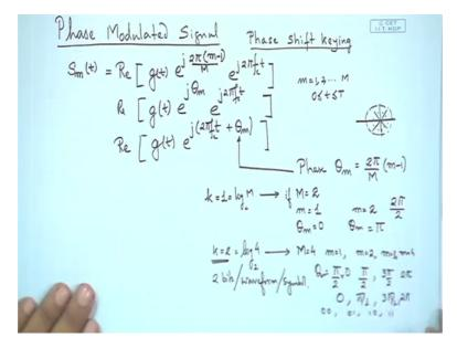
So, at this point we would like to move over to the discussion of the next modulation technique which comes under the category of phase modulation or phase modulated signal you can say right and rather we could call this a phase shift keying, because there is a more appropriate term as will be clear like in the previous case we would call amplitude shift keying here we would call it the phase shift keying.
