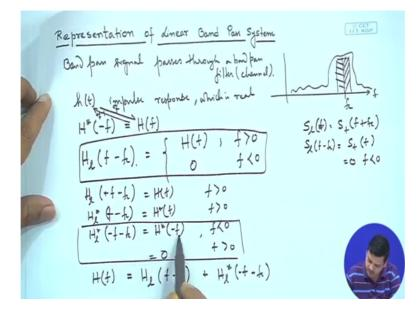
So that means, this thing is nearly 0 for f less than 0 and this thing is nearly 0 for f negatives similarly if we go by the definition of h of f, what you have over here. What we see is that this is H f for f greater than 0, 0 for less than 0 and this quantity is 0 for f greater than 0. So, we could we could say at this is almost equal to 0 for f greater, than 0 this is almost equal to 0 for f less than 0 in a same manner.
