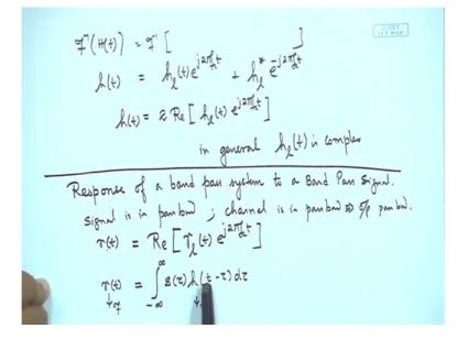
So, output r t is a convolution of S t and h t. And if we take the Fourier relationship it turns out to be this.
